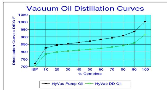
HyVac Direct Drive Oil is also high boiling range, straight mineral oil of approximately 200 SUS at 100° F. Its low vapor pressure and other unique characteristics make it especially suitable for use in most direct drive mechanical vacuum pumps employing hydrocarbon based pump fluids including Welch, Leybold, Edwards, Alcatel, Precision, HyVac 30L and HyVac 55L pumps.
