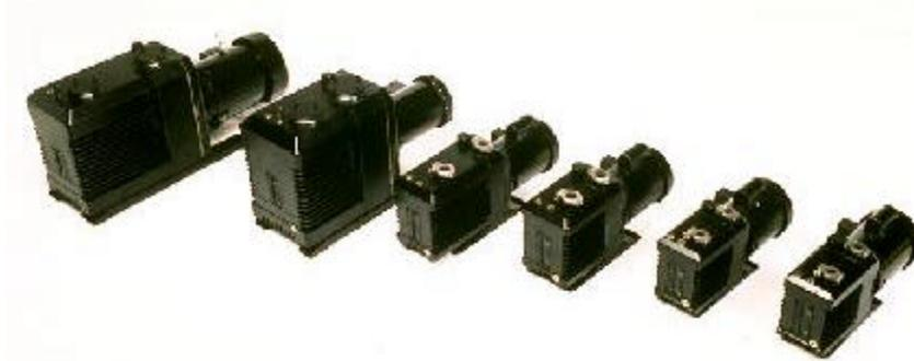
These six mechanical high vacuum pumps are the newest addition to the HYVAC line. They incorporate two stage design, with the basic oil sealed rotary vane principle. They are excellent general purpose or roughing pumps capable of vacuum pressures to  $5 \times 10^{-4}$  Torr or .5 micron with fast recovery times. Since they are direct drive pumps, they offer high volumetric efficiency with ease of portability.
