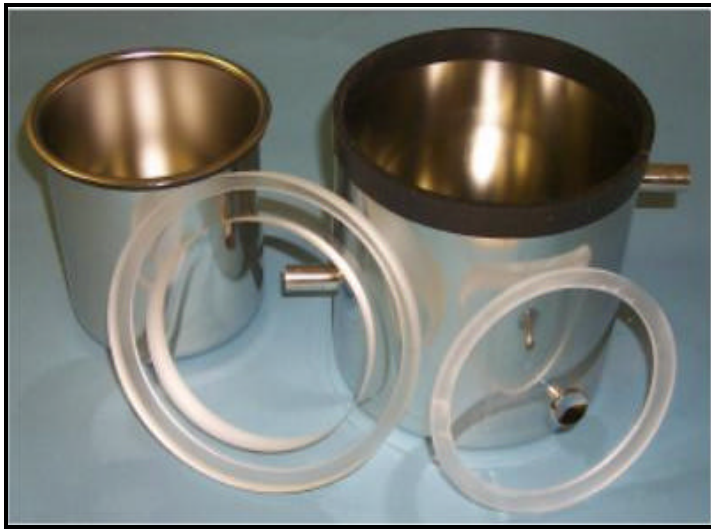
Pictured - 3/4" Hose connections on DIT DIT apart
